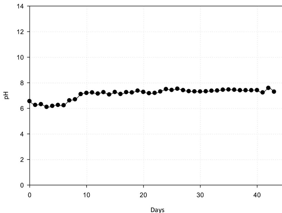
Fig. 3. pH of the bioreactor during the batch operation of the lab scale anaerobic digester. For the batch operation of the bioreactor the feedstocks and the inoculum were added at once during start-up.
